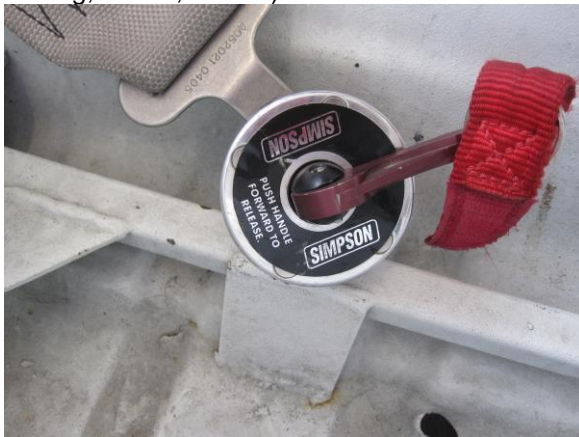
Over-center latch originated with the aircraft Industry but have been adapted for racing. This over-center may be five or six point Attachment.
