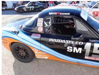
Symbol on body is adjacent to the switch just inside the window.
