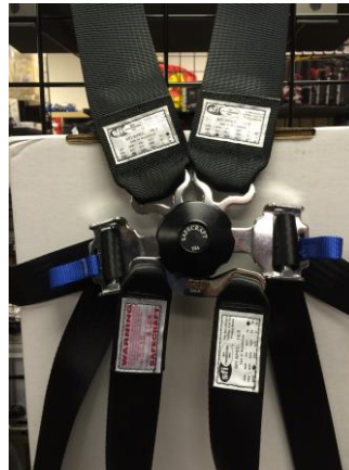
A six point harness with two straps between the legs. This Safecraft harness also released with a rotary motion of the central cover. (Safecraft picture courtesy of Winding Road Racing, Austin, Texas.)
