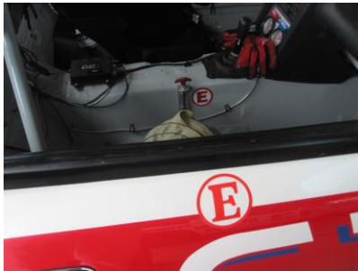
Symbol on door with fire Extinguisher on console
