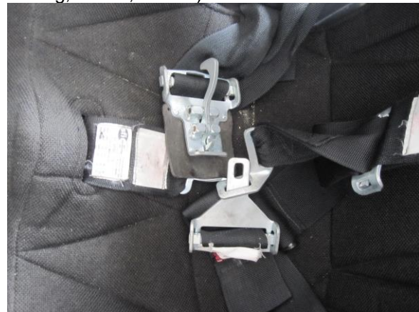
This older style of over-center is usually found with Five point attachments. Note that belts are linked prior to being secured.
